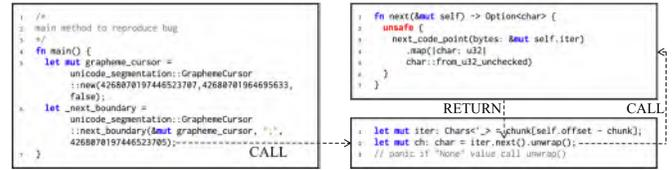
**Figure 5: Code to reproduce bug in unicode-segmentation**
