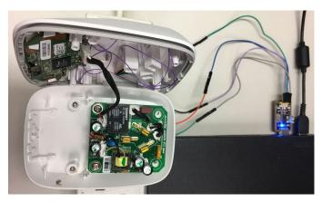
Fig. 6: The Belkin Wemo Switch. The debugging ports on the motherboard is connected to a computer with a serial to USB converter
