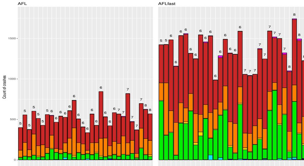
**Figure 6: Crashes with unique bugs found per run for *cxxfilt*. Each bar represents an independent run of either AFL or AFLfast. The height of the bar is the count of crashing inputs discovered during that run. Each bar is divided by color, clustering inputs with other inputs that share the same root cause. Number of unique bugs is indicated above each bar.**
