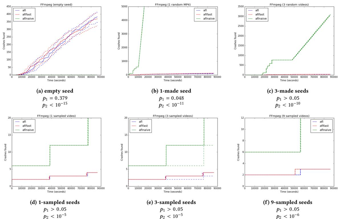
Figure 3: *FFmpeg* results with different seeds. Solid line is median result; dashed lines are confidence intervals.  $p_1$  and  $p_2$  are the p-values for the statistical tests of AFL vs. AFLFast and AFL vs. AFLNaive, respectively.
